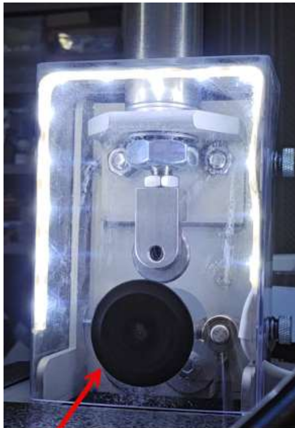
New removable plug for chopping longer cane safely.
